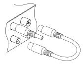
Connect the antenna cable to the ANT 1 socket on the back panel of the digital receiver.
